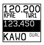
When dual watch is enabled, the SkyView Com Radio monitors the standby frequency for transmissions while simultaneously monitoring the active frequency, allowing you to listen to both (but not simultaneously). This allows you to listen to ATIS on standby, for example, while keeping tower tuned to the active frequency.
