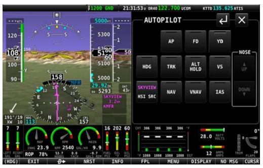
Figure 231 – AUTOPILOT Control page – Expert Control Scheme
