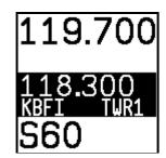
Use the TWR, ATIS, GND, and ATC buttons on the control panel to send the associated airport frequencies to the standby frequency location:
