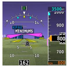
Figure 37 – MIN Bug and "MINIMUMS" Alert
