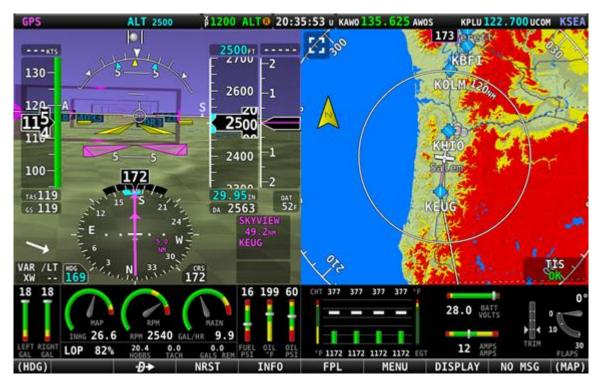
Figure 14 – 50% PFD / 50% MAP with ENGINE BOTTOM BAND
