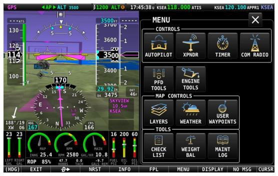
Figure 17 – ENGINE BOTTOM BAND partial over-written by MENU page
