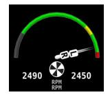
Figure 201 – Example of a Synchroscope and a Combined RPM Widget
