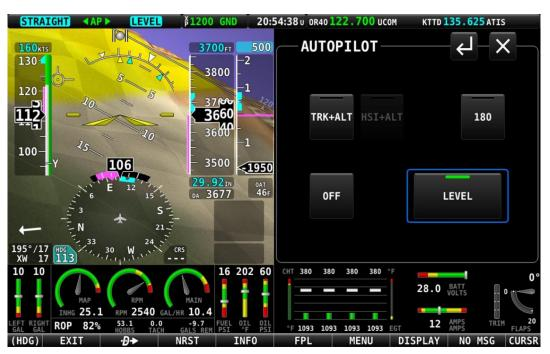
Figure 228 – LEVEL mode is engaged
