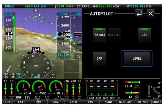
Figure 227 – 180° mode is engaged; turn is not yet complete
