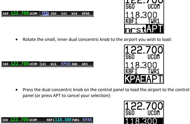
Use the TWR, ATIS, GND, and ATC buttons to send the associated airport frequencies • to the standby frequency location:
