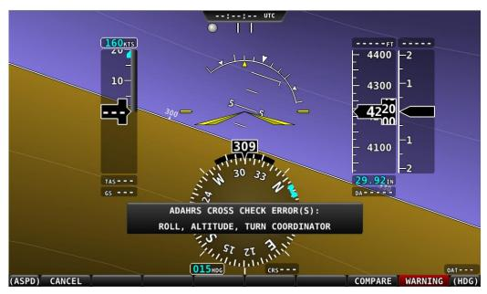
Figure 87 – ADAHRS Cross-Checking Disagreement
