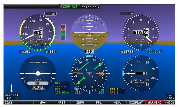
Figure 76 – Six Pack PFD Presentation, Synthetic Vision Enabled
