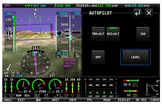
Figure 226 – HSI+ALT mode is engaged
