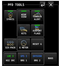
Figure 51 Bearing Pointer Selector in PFD TOOLS
