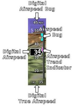
Figure 31 – Example Airspeed Indicator
