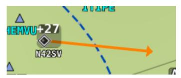
Figure 122 – Traffic Targets Display of Tail Numbers
