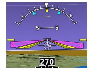
Figure 234 – Single Cue / Inverted-V with Autopilot Servos Not Engaged
