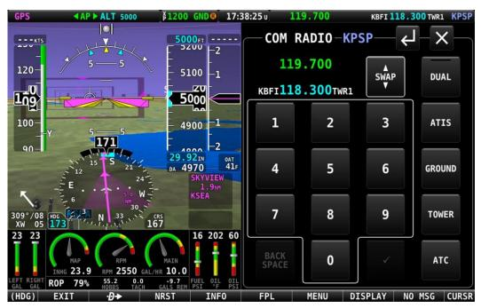
Figure 242 – Com Radio Control Panel
