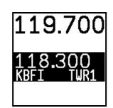
• With a valid Com frequency highlighted, (a 25kHz frequency on the SV-COM-X25 and SV-COM-C25 and an 8.33kHz on the SV-COM-X83) press the TUNE COM button to send the frequency to the standby frequency:
