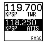
The squelch setting, which determines how strong a radio transmission must be before the radio receives it, is configured during setup. See the *SkyView Classic / SE / HDX System Installation Guide* for instructions on adjusting this parameter.
