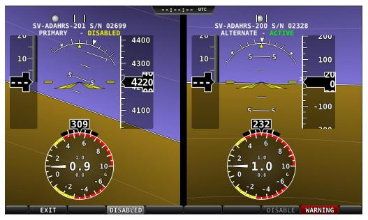
Figure 89 – ADAHRS Cross-Check Comparison (one ADAHRS disabled)
