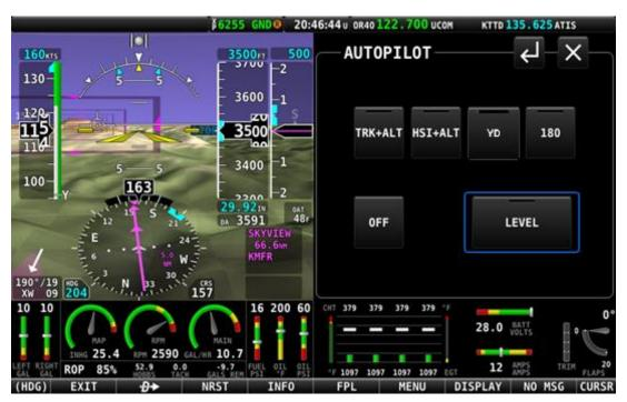
Figure 224 – AUTOPILOT Control page – Simplified Control Scheme
