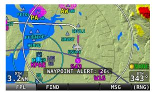
Figure 158 – Flight Plan Alert Messages
