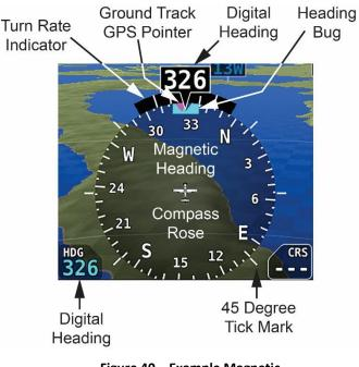
Figure 40 – Example Magnetic Heading Indicator/Directional Gyro
