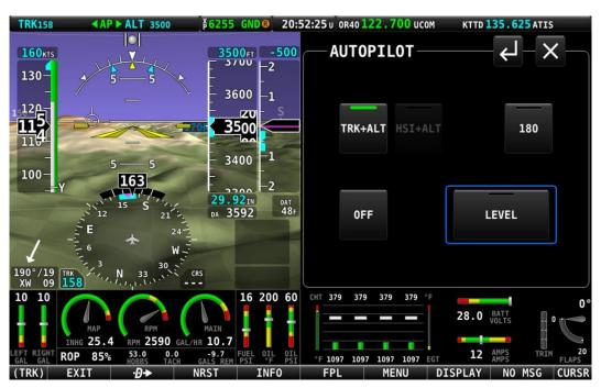
Figure 225 – TRK+ALT mode is engaged
