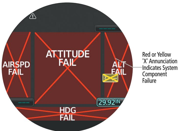
Example of Failure Annunciations
