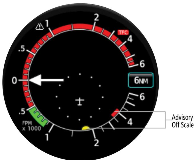
If a TA or an RA intruder does not have a bearing, it will be displayed at a textual alert across the top portion of the traffic display. All textual TA's or RA's are in the format (alert type) (distance in nm) (relative altitude in hundreds of feet) (climbing or descending arrow, if applicable). The text is colored red (RA) or yellow (TA) based upon the alert type.
