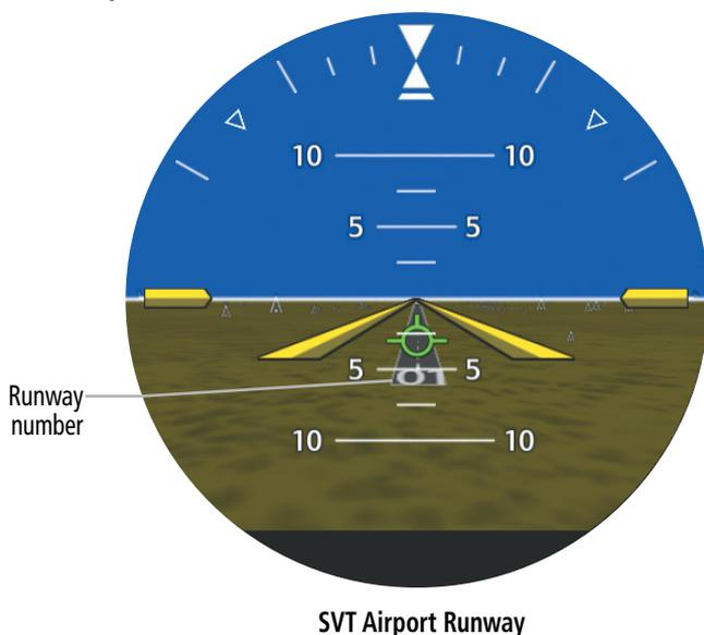
**WARNING:** Do not use the Garmin SVT runway depiction as the sole means for determining the proximity of the aircraft to the runway or for maintaining the proper approach path angle during landing.
