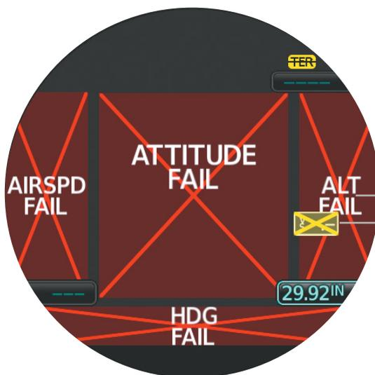
Failure Annunciators Example
